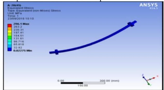
Fig. 3: Equivalent stress of shaft, Mpa
