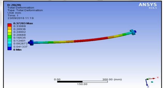
Fig. 4: Total deformation of shaft in mm.
