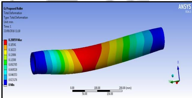
Fig. 8: Total deformation of roller in mm.
