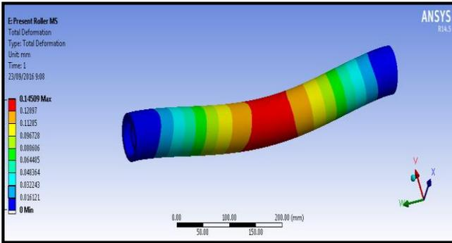
Fig. 6: Total deformation of roller in mm
