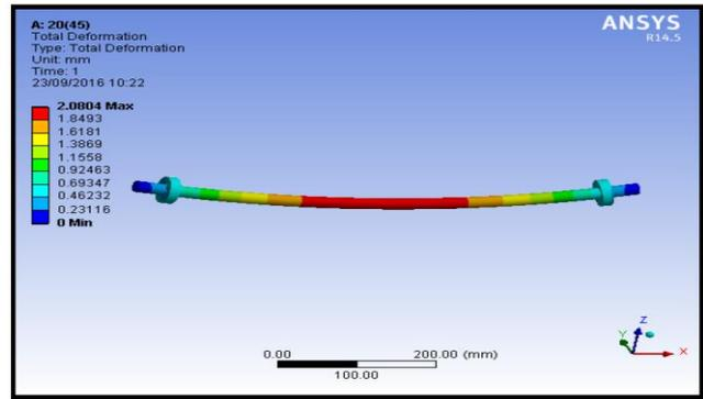
Fig. 2: Total deformation of shaft in mm.
