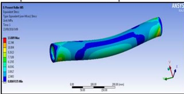
Fig. 7: Equivalent stress of roller, Mpa
