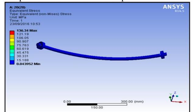
Fig. 5: Equivalent stress of shaft, Mpa
