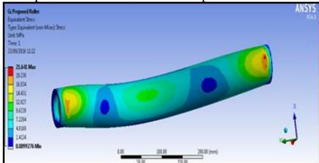
Fig. 9: Equivalent stress of roller, Mpa
