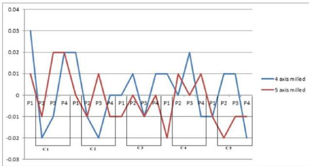
Fig. 9: Comparison of deviation of crown copings milled with 4-axis and 5-axis milling machine.
