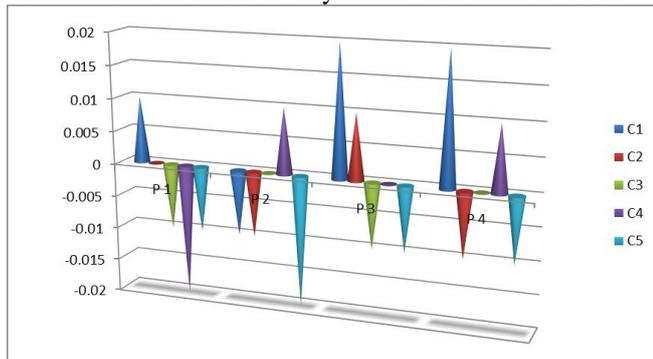
Fig. 8: Graph of deviation for 5-axis milled crowns.
