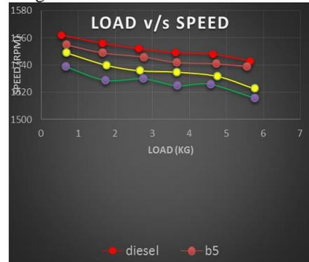
Fig. 4: Load v/s Speed
