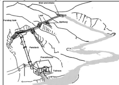
Fig. 2: Different Components of the Small Hydro Power Plant
