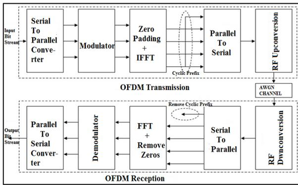
Fig. 3: Block Diagram of OFDM system
