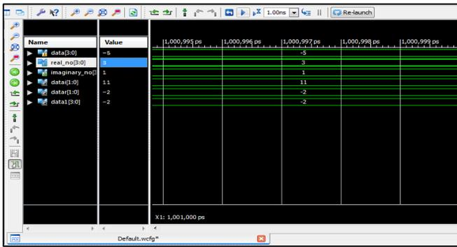
Fig. 6: Simulation result of 16-QAM modulator
