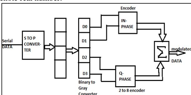
Fig. 4: 16-QAM Block Diagram
