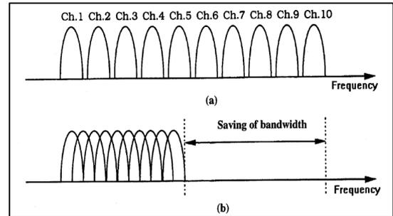
Fig. 1: (a) Spectrum of FDM showing guard bands (b) Spectrum of OFDM showing overlapping subcarriers
