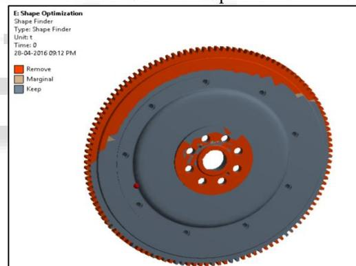
Fig. 16: Optimization result for Al Alloy Flywheel.
