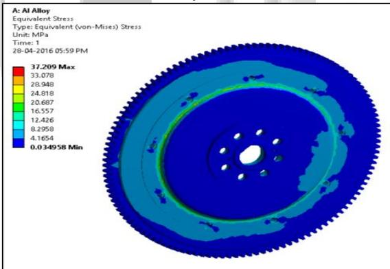
Fig. 6: Radial stress developed in Al 6063 T6 flywheel
