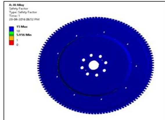
Fig. 8: Factor of safety of Al 6063 T6 flywheel.
