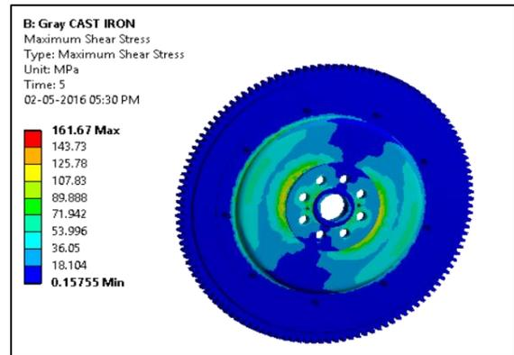
Fig. 15: Shear stress developed in Gray CI flywheel.
