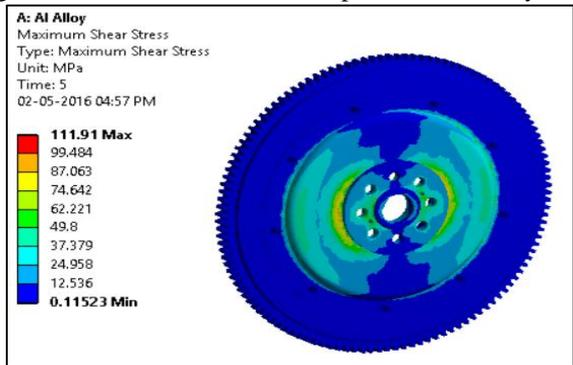
Fig. 12: Shear stress developed in Al 6063 flywheel.
