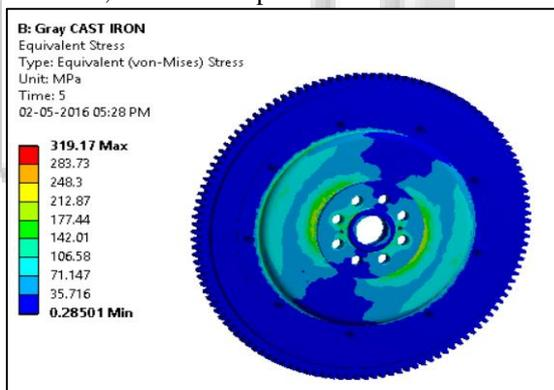
Fig. 13: Non-Linear Radial stress developed in Gray CI flywheel.
