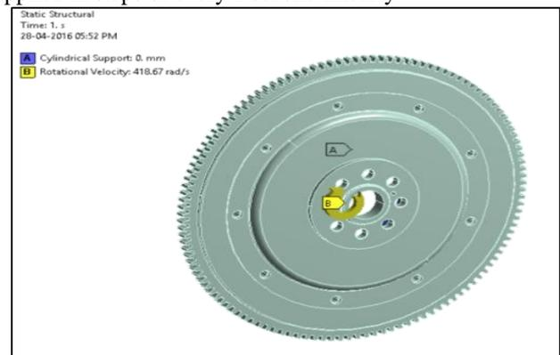
Fig. 3: Boundary Condition on Flywheel
