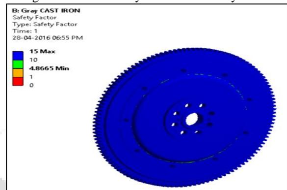
Fig. 9: Factor of safety of cast alloy flywheel.
