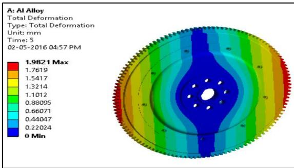
Fig. 11: Total Deformation developed in Al 6063 flywheel.
