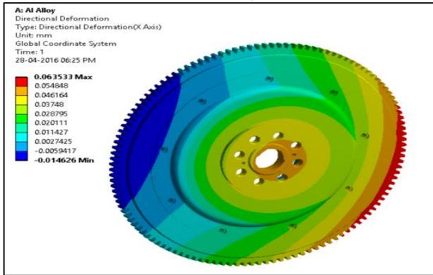
Fig. 4: Radial deformation of Al 6063 T6 flywheel.
