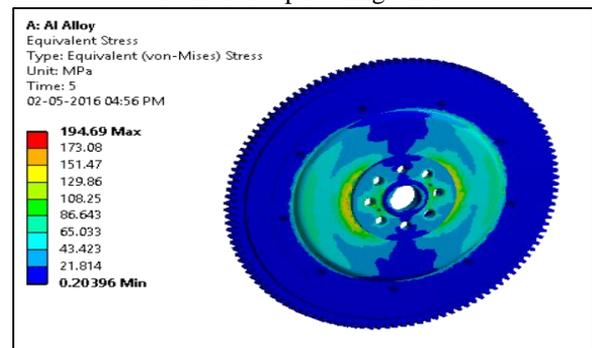
Fig. 10: Non-Linear Radial stress developed in Al 6063 flywheel.
