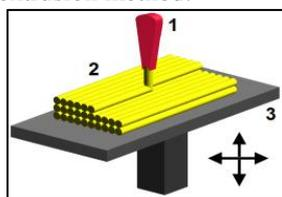
Fig. 2: Process of 3-D Printing
