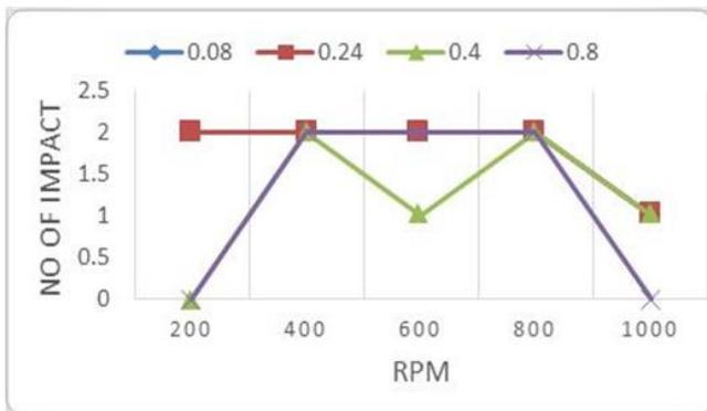
Fig. 9: Variation of rpm with Number of Impacts of damper for 0.08 mm, 0.24mm, 0.4 mm and 0.8 mm clearance
