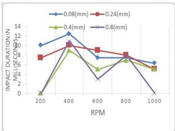
Fig. 10: Variation of rpm with Impact Duration of damper mass 3 percent of main mass for 0.08 mm, 0.24mm, 0.4 mm and 0.8 mm clearance
