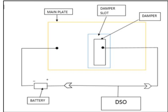
Fig. 5: Schematic block diagram of damper connection
