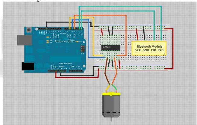
Fig. 2: Motor control connection
