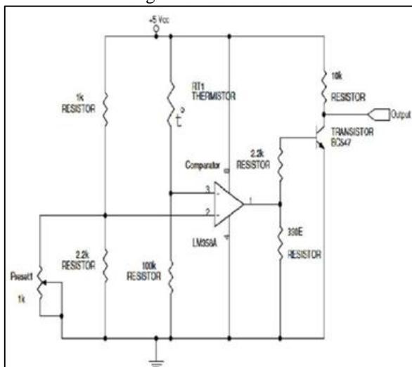
Fig. 5: Circuit diagram for temperature sensor
