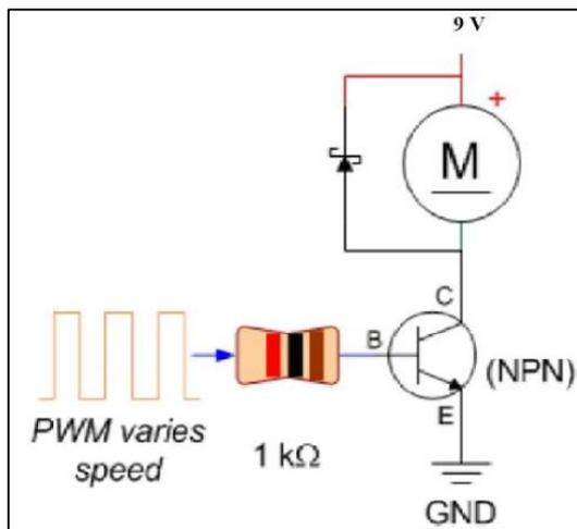
Fig. 3: Driver circuit
