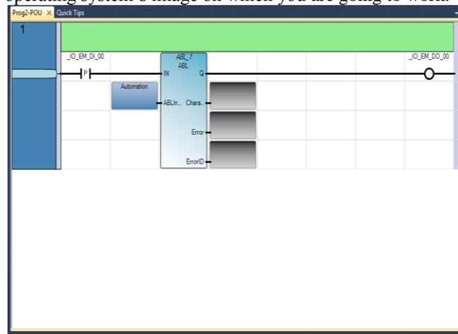
Fig. 2: Program for storing any input string length in the buffer of the plc
