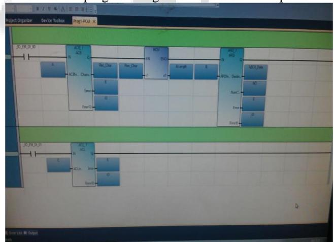
Fig. 4: Program for reading characters from plc to pc i.e. HyperTerminal
