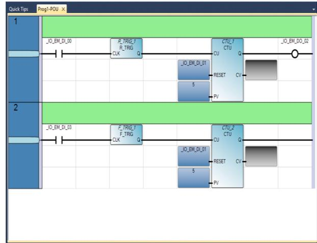
Fig. 3: Program for counting the number of pulses.
