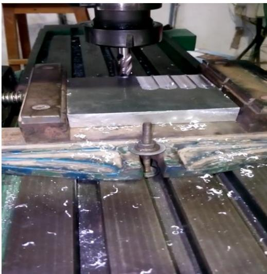
Fig. 1: End Milling Operation
