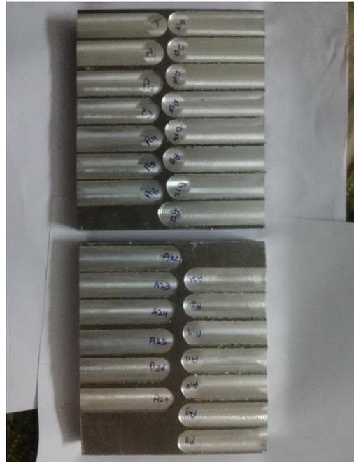
Fig. 2: Workpieces after machining by HSS end mill
