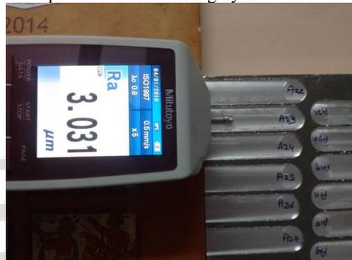
Fig. 3: Surface roughness measurement
