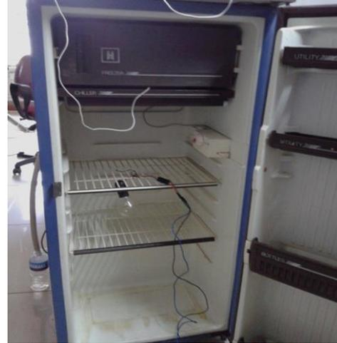
Fig. 4: A view of refrigerator with bulb placed inside the cabin for load performance
