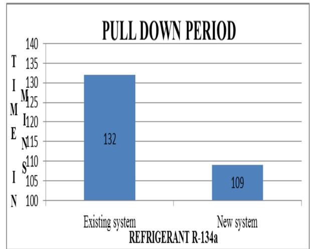
Fig. 9: Pull down period for refrigerant R-134a
