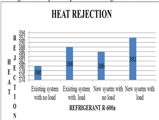
Fig. 13: Heat rejection for refrigerant R-600a
