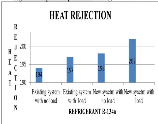
Fig. 8: Heat rejection for refrigerant R-134a
