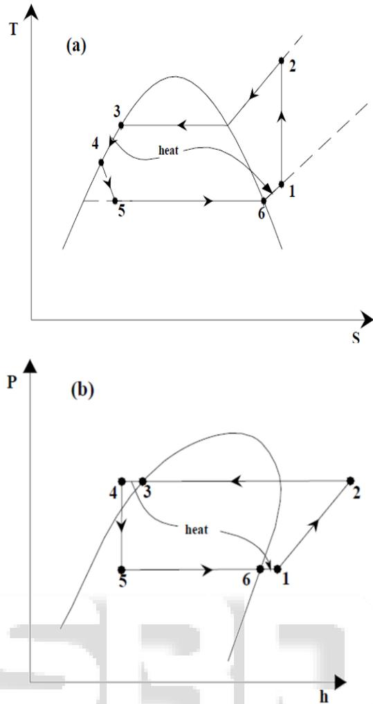
Fig. 2: VCRS cycle with LSHX (a) on T-S diagram (b) on P-h diagram
