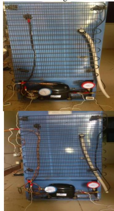
Fig. 3: a) Existing System and b) New system with 35cm length of heat exchanger
