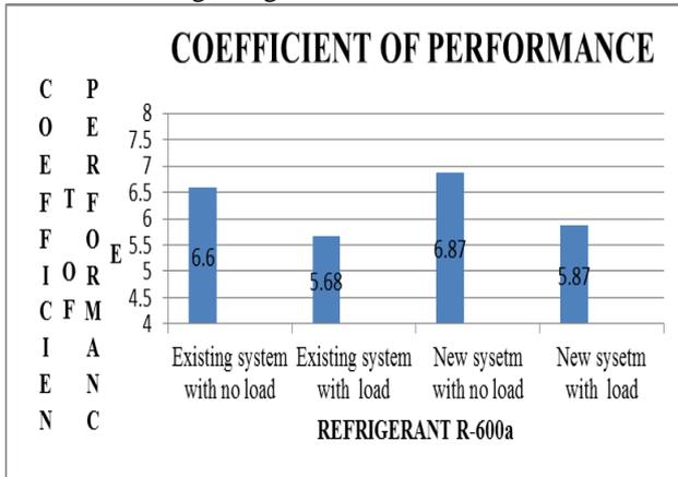
Fig. 11: Coefficient of performance for refrigerant R-600a
