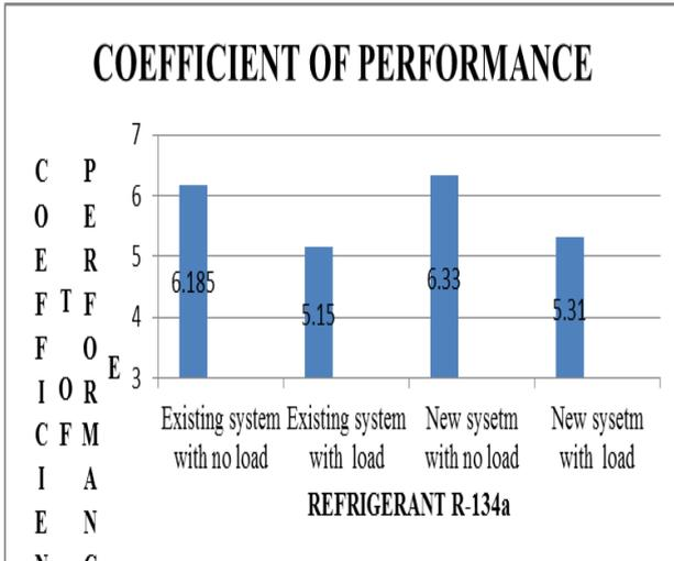
Fig. 6: Coefficient of performance for refrigerant R-134a
