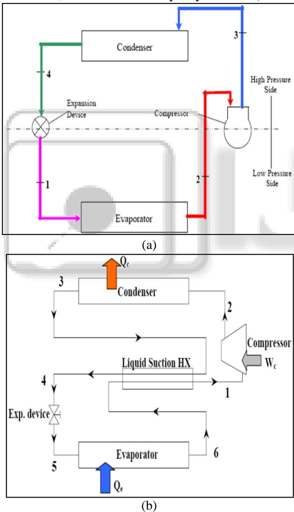
Figure1 Schematic of hardware arrangements for a) The basic cycle and b) Cycle with the liquid line-suction line heat exchanger
