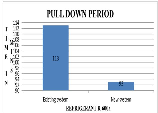
Fig. 14: Pull down period for refrigerant R-600a
