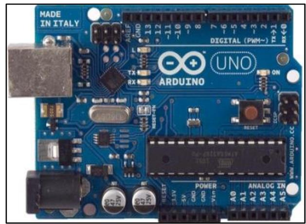
Fig. 4: Arduino uno Development Board
