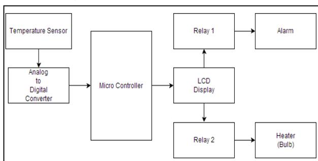
Fig. 2: Block Diagram of Radiant Warmer
