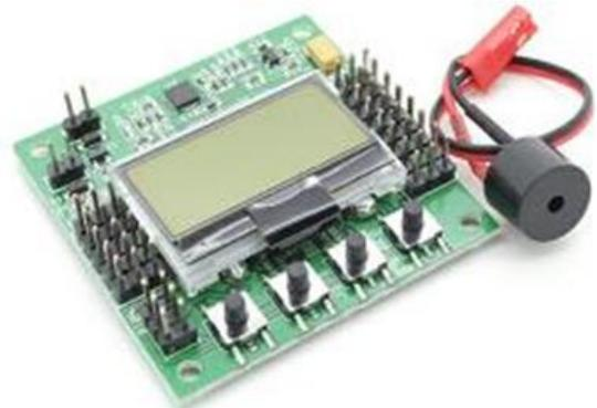
Fig. 3: Flight Controller
