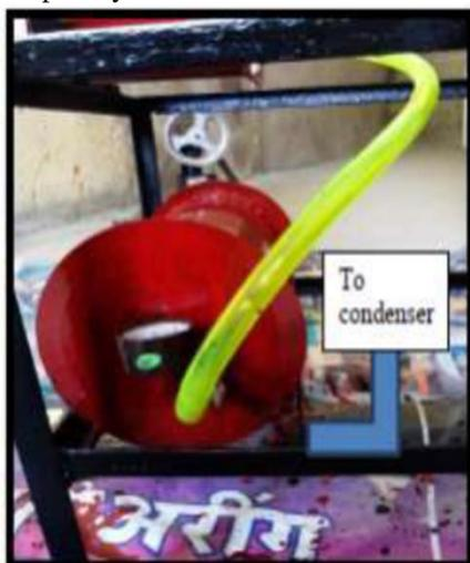
Fig. 3: Connection of Receiver to Condenser
