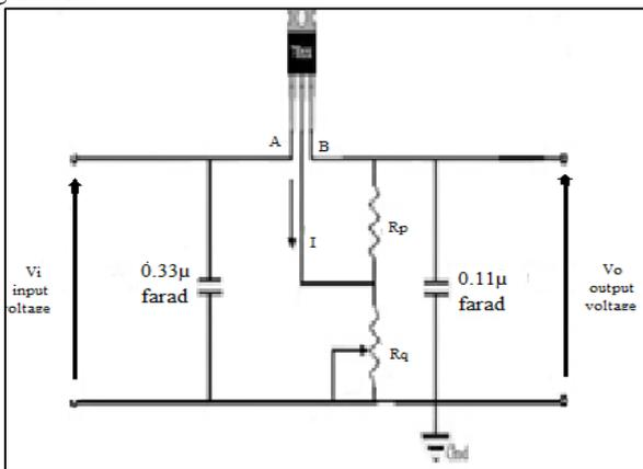
Fig. 1: Voltage Regulator Circuit
