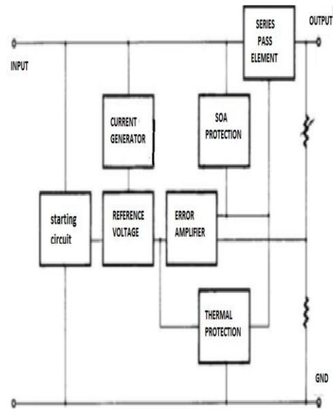
Fig. 2: Block Diagram of Voltage Regulator
