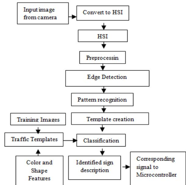
Fig. 3: Image processing block diagram
