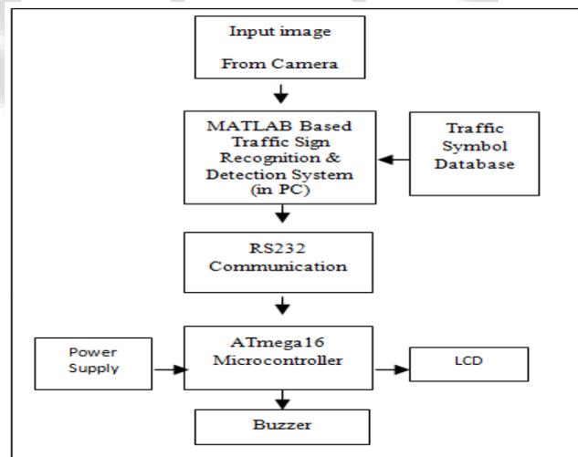
Fig. 1: Main system block diagram
