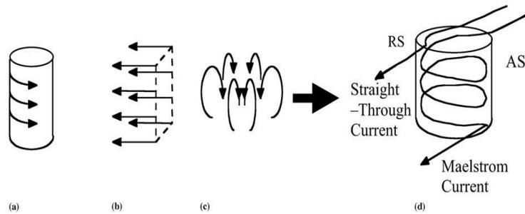
Fig. 2.3: Deconvolution Of Fsw Process Of Three Flow Fields Into Two Flow Currents (a) Rigid body motion (b) Uniform translation (c) Ring vortex (d) Two flow currents: Advancing side and Retreating side<sup>[18]</sup>
