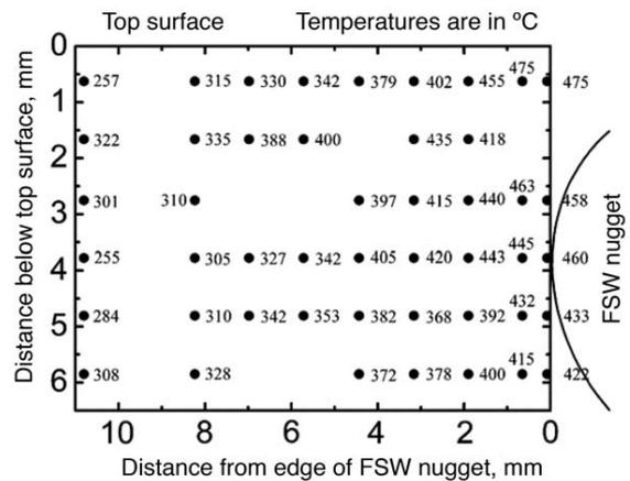
Fig. 2.1: Temperature Distribution Observed<sup>[18]</sup>
