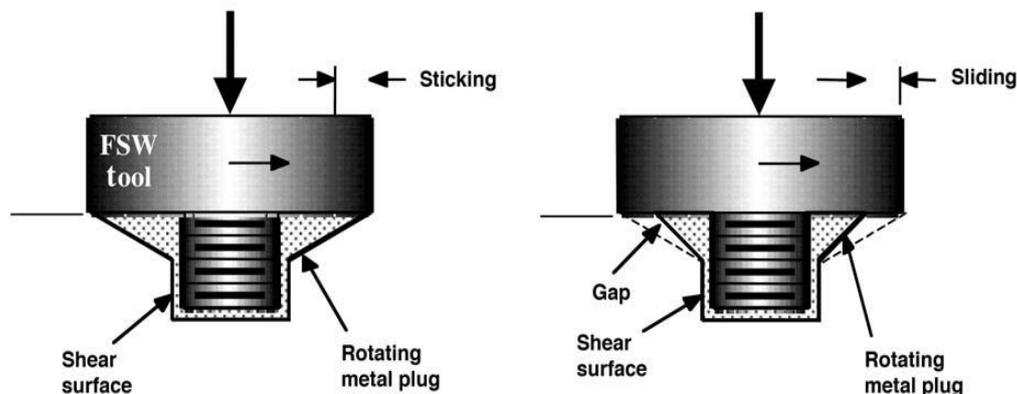
Fig. 2.2: Alternating (Stick Slip) Boundary Conditions At The Interface<sup>[18]</sup>
