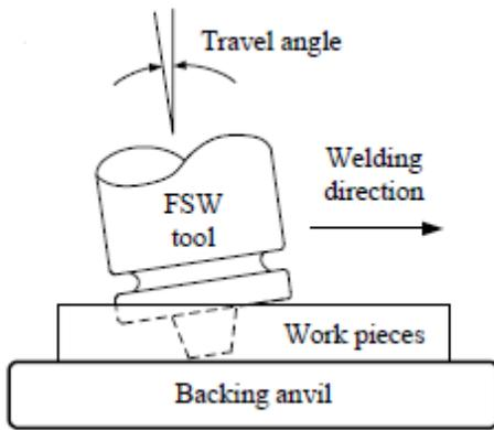
Fig. 1.2(a): Travel Tilt Angle Used In FSW<sup>[4]</sup>
