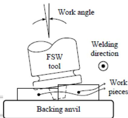
Fig. 1.2(B): Work Tilt Angle Used In FSW<sup>[4]</sup>
