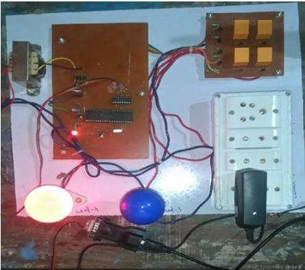
Fig. 4: Embedded system to control load
