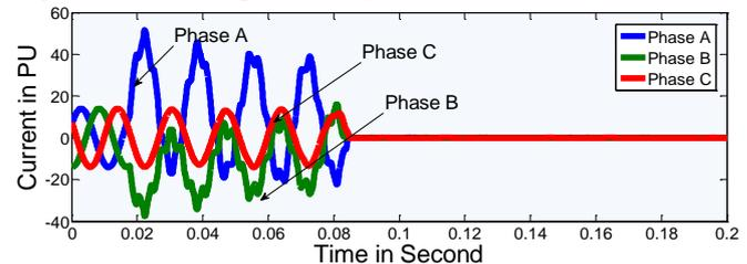
Fig. 5: Current Response of System for LL fault (phase AB)
