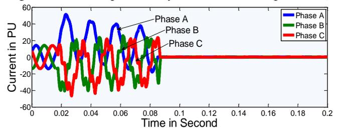
Fig. 6: Current Response of System for LLL fault (Phases ABC)
