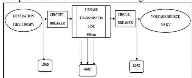
Fig. 1: Block Diagram of proposed scheme
