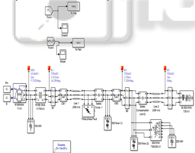
Fig. 3: Simulation model of three phase transmission line
