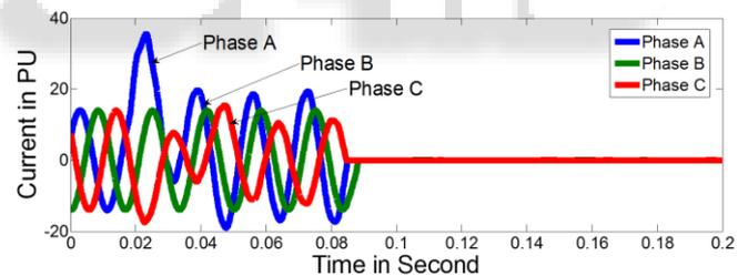
Fig. 4: Current Response of System for SLG Fault (Phase A)
