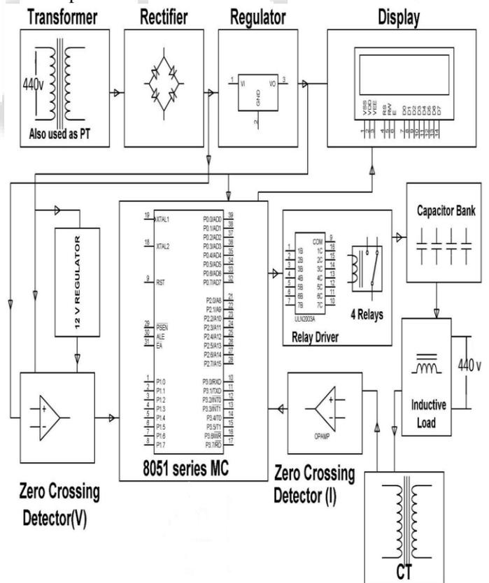
Fig. 1: block diagram of APFC unit
