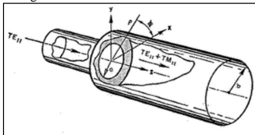
Fig. 1:  $TE_{11} \rightarrow TM_{11}$  mode conversion at discontinuity in circular waveguide<sup>[3]</sup>.
