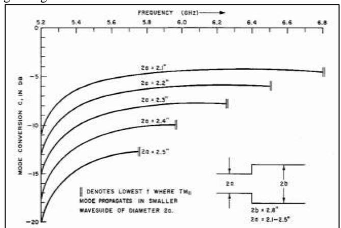
Fig. 3:  $TE_{11} \rightarrow TM_{11}$  mode conversion coefficient at step discontinuity<sup>[3]</sup>.
