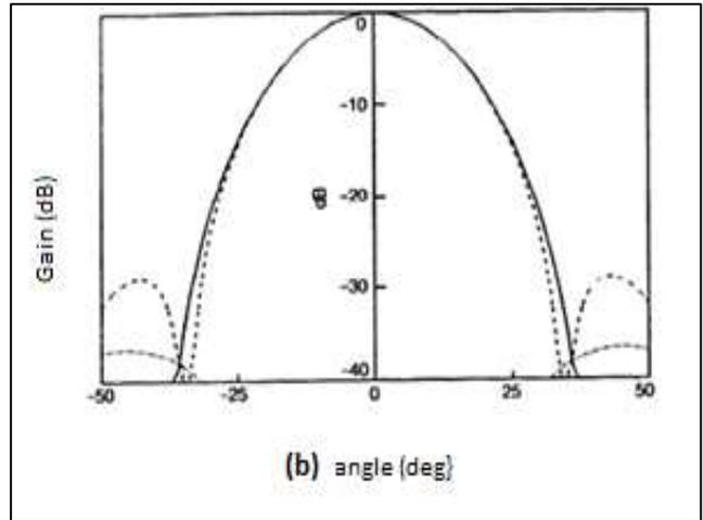
Fig. 5: Radiation pattern (Gain) of dual mode waveguide (a) TE<sub>11</sub> mode alone, (b) TE<sub>11</sub> + 5% TM<sub>11</sub> mode [2]
