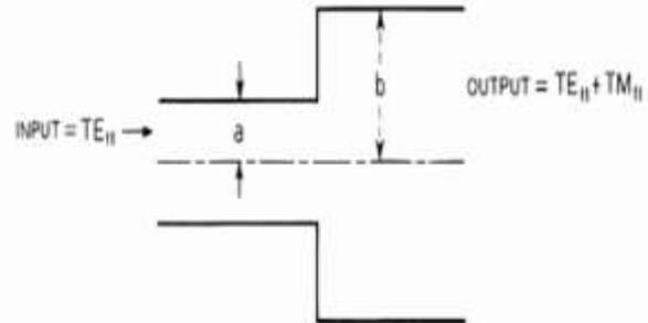
Fig. 2: Mode conversion at step discontinuity by changing radius of waveguide<sup>[3]</sup>.
