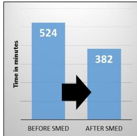
Fig. 8: Comparison Between Before Implementation and after Implementation of SMED
