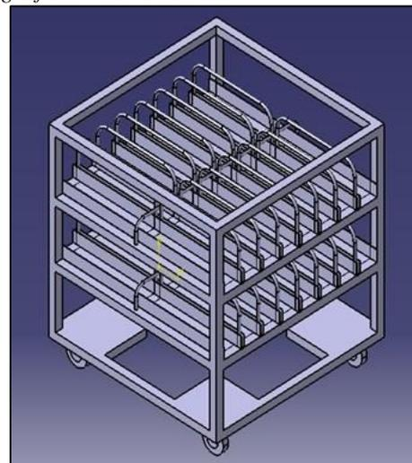
Fig. 5: CAD Model of Trolley for Oil Lube Cooler
