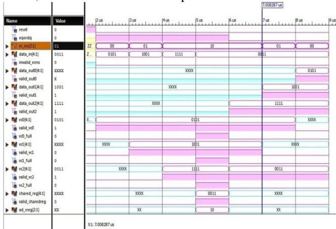
Fig. 5: Output Waveforms for 3VC elastistore Architecture with 4 bits data.
