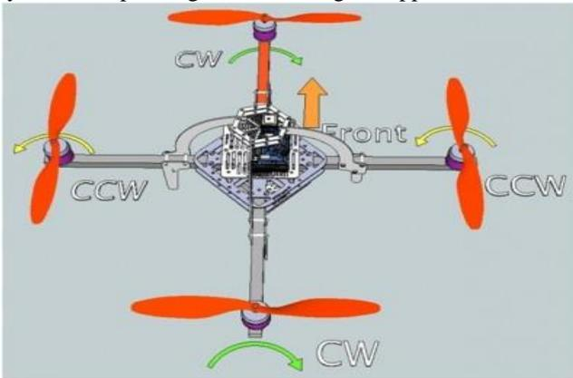
Fig. 2: Quad copter motor configuration
