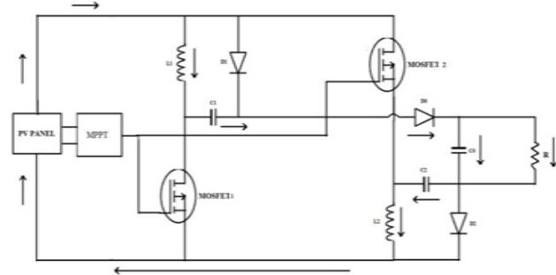
Fig. 6: When both the switches are off
