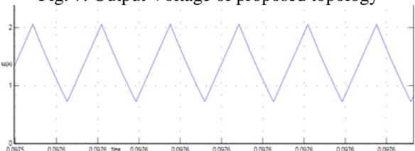
Fig 8: Inductor current through L1
