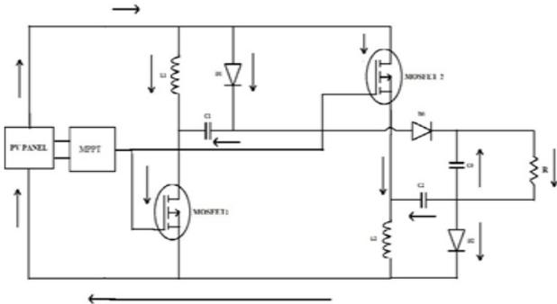
Fig. 5: When both the switches are on
