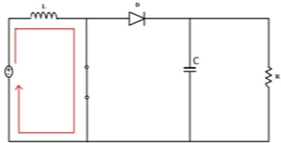
Fig 2: Switch is on
