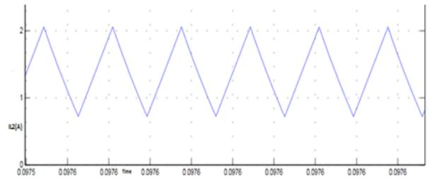
Fig. 9: Inductor current through L2
