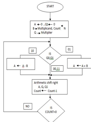
Fig. 2: Flowchart for booth's algorithm of signed number
