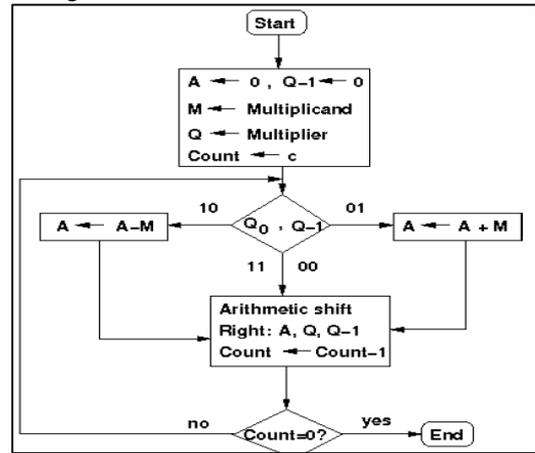
Fig. 4: Design flow of Booth algorithm
