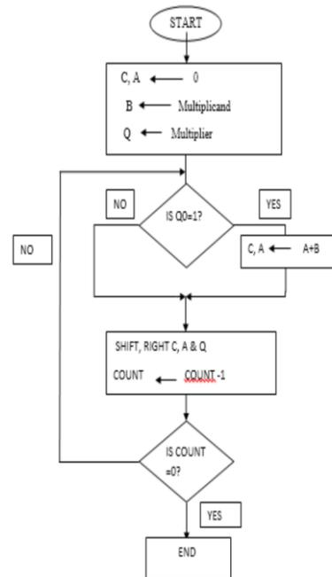
Fig. 1: Flowchart for booth's algorithm of unsigned number
