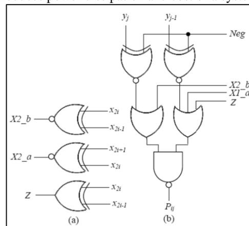
Fig. 5: The Encoder and Decoder for the new MBE scheme.
