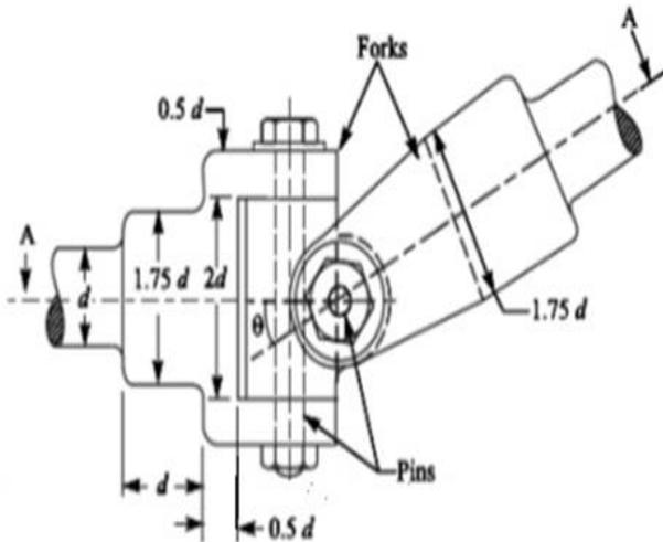
Fig. 4: Double Universal Joint
