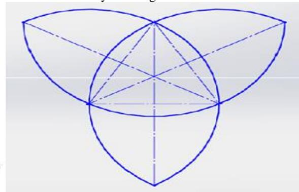
Fig. 2: Construction of Reuleaux triangle
