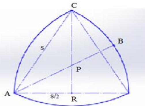
Fig. 3: Geometrical construction of Reuleaux triangle
