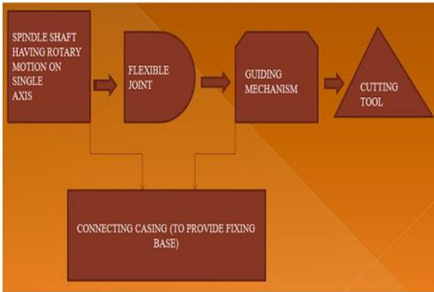
Fig. 8: Block Diagram of whole mechanism
