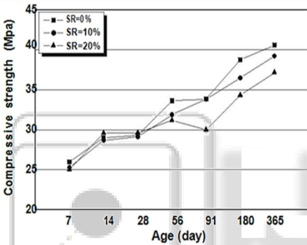
Fig. 2: Relationship between compressive strength and age with SR.
