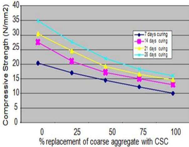
Fig. 1: Compressive strength of CSC of mix proportion 1:1:2
