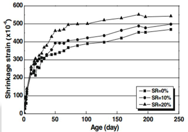
Fig. 5: Influence of SR on shrinkage strain
