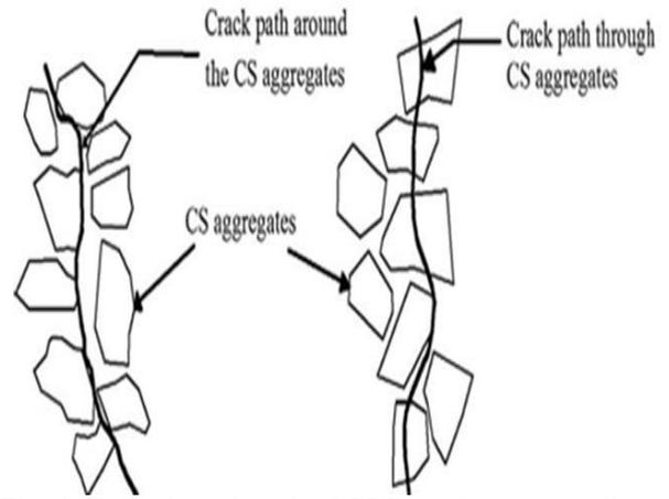
Fig. 4: Typical crack path of CSC specimens at earlier and at later age
