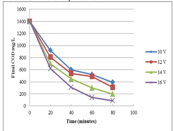
Fig. 4: Effect of Voltage on COD
