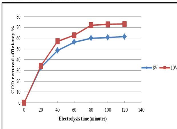
Fig. 2: Effect of Electrolysis Time at pH 9
