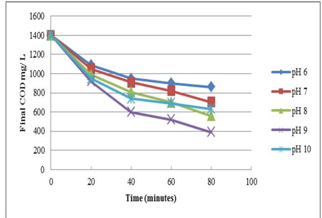
Fig. 3: Effect of pH at 10V
