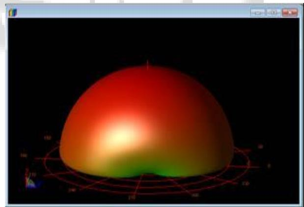
Fig. 8: 3D Radiation pattern of Yagi patch with one Reflector at S band
