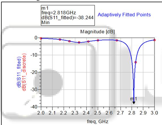
Fig. 6: Graph of Return loss of RReflector schematic
