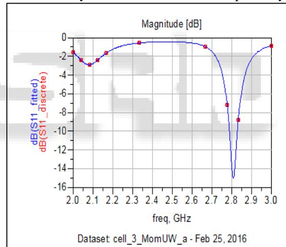
Fig. 3: Graph of Return loss of patch
