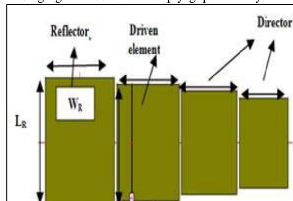
Fig. 1: Microstrip Yagi patch antenna
