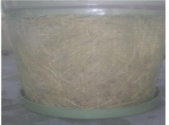
Fig. 11: Bamboo pad material in evaporative coolers
