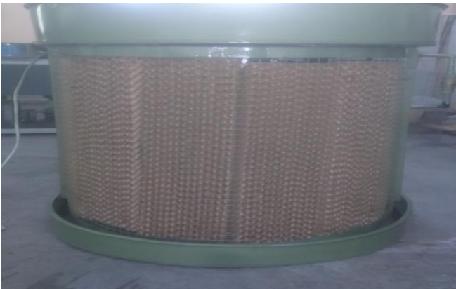
Fig. 9: Celdek as a cooling pad in evaporative cooler Result obtained from experiment performed with Celdek is as given below in table 2.
