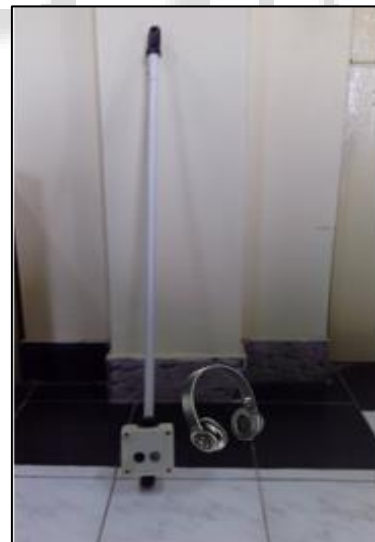
Fig. 6: A Blind Stick with the wireless Bluetooth headset
