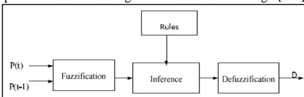
Fig. 3: Block Diagram of Fuzzy logic Controller
