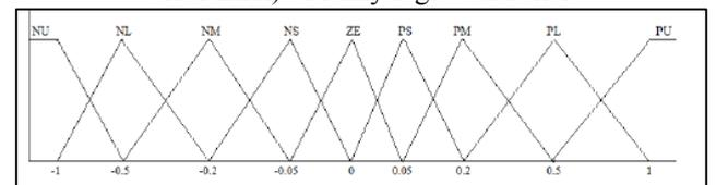
Fig. 6: Output membership function (delta D) of fuzzy logic controller
