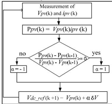
Fig. 2: Algorithm of P & O method for the MPPT
