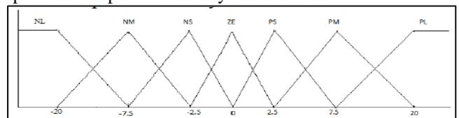
Fig. 5: Input membership function (error ER and change error delta ER) of fuzzy logic controller
