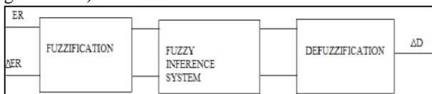
Fig. 4: configuration of fuzzy controller for MPPT
