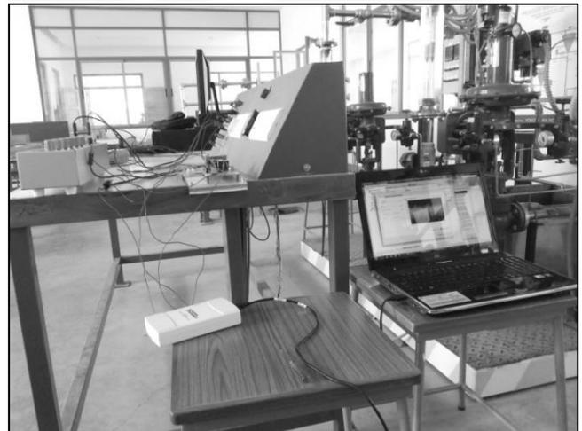
Fig. 4: The experimental setup of pneumatic actuator fault diagnosis
