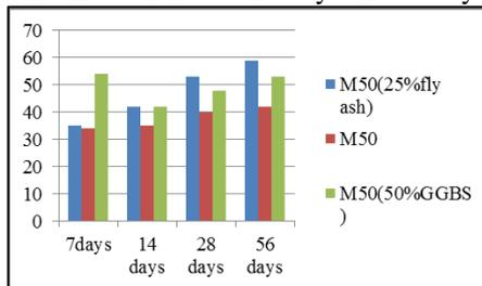
Fig. 6: Sea water mixing and normal water curing
