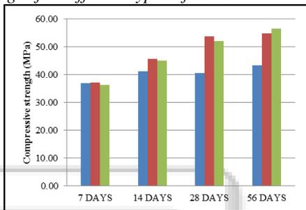
Fig. 9: Normal water mixing in M50 and sea water curing
