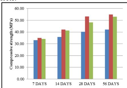
b) For Sea water mixing and normal water curing of M30, M40 and M50
