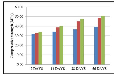
Fig. 11: Sea Water mixing in M50 and Sea Water curing
