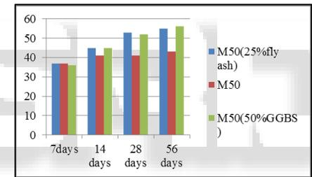
Fig. 5: Normal water mixing and sea water curing
