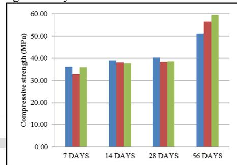
Fig. 12: Normal water mixing and curing in M50
