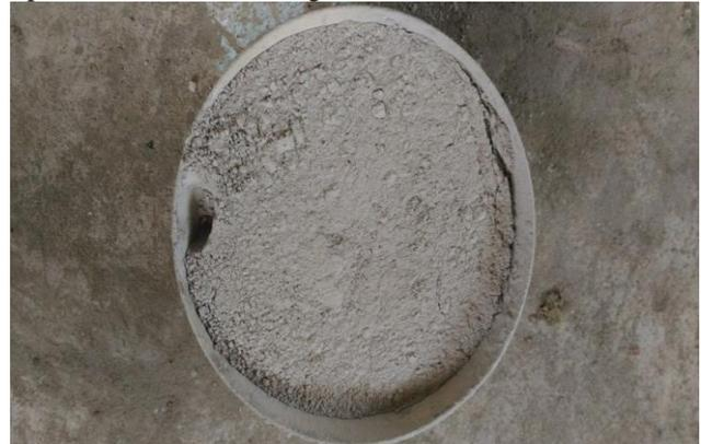
Fig. 2: Ground Granulated Blast Furnace Slag
