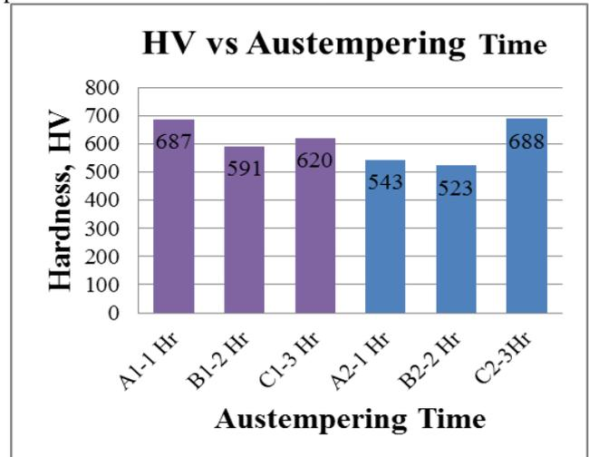
Fig. 5: Comparative graph of Micro-Hardness.
