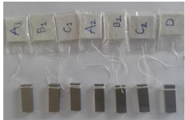
Fig. 1: CADI Samples prepared for Salt Spray Fog test.
