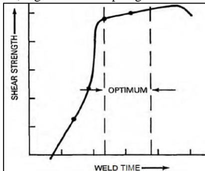
Fig. 4: Tensile-shear strength as a function of weld time
