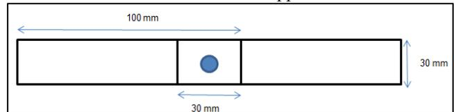
Fig. 5: Tensile shear test sample
