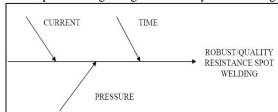
Fig. 2: Cause and effect diagram of main welding parameters
