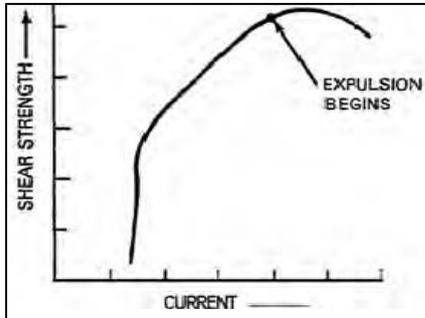
Fig. 3: Effect of welding current on spot weld shear strength
