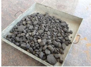
Fig. 1: coal washery reject
