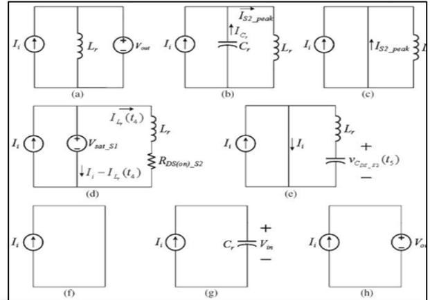
Fig. 2: Equivalent circuits during one switching cycle
