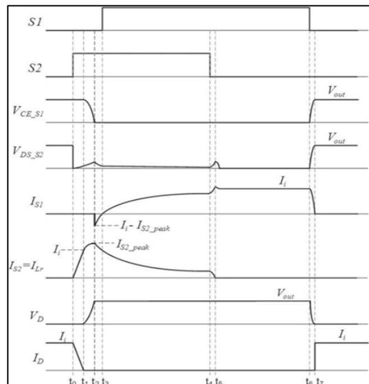
Fig. 3: Theoretical waveforms of the proposed ZVT-PWM boost converter
