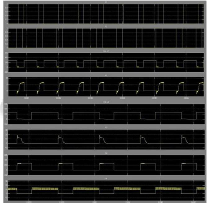
Fig. 6: Simulation waveforms for the proposed ZVT-PWM boost converter
