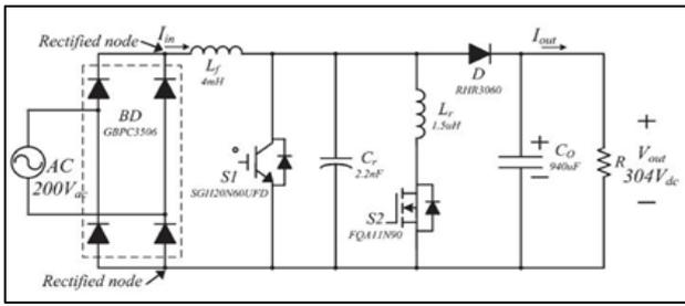
Fig. 4: Proposed ZVT-PWM boost converter.
