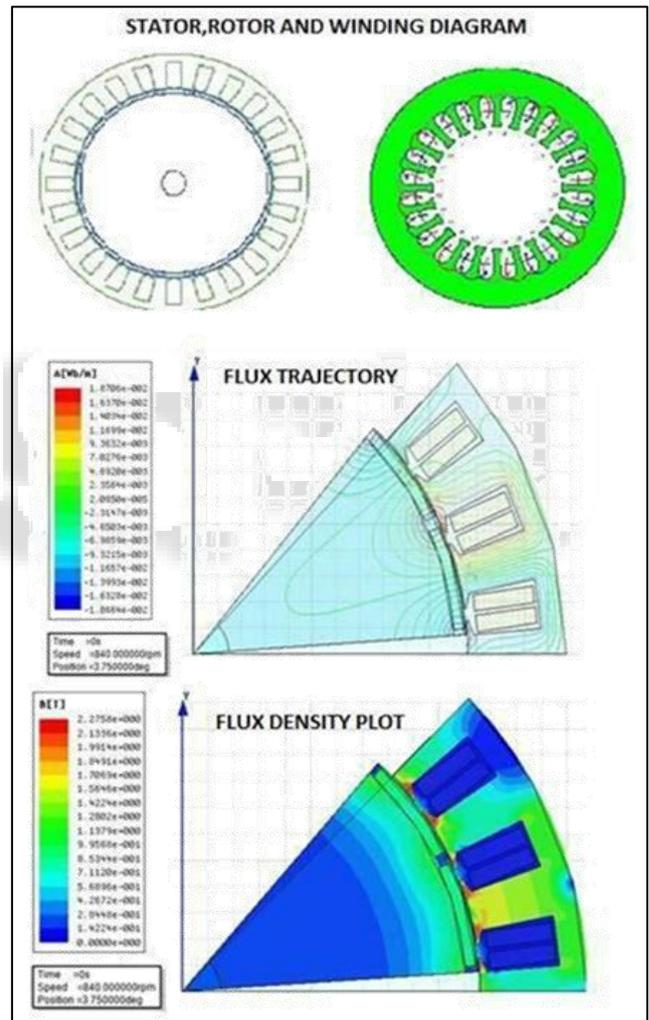
Fig. 4: Finite Element Analysis Plot of PMSM
