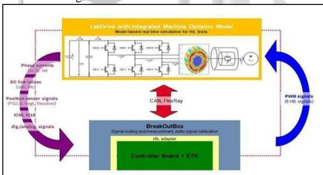
Fig. 8: HIL Module with integrated dynamic machine model
