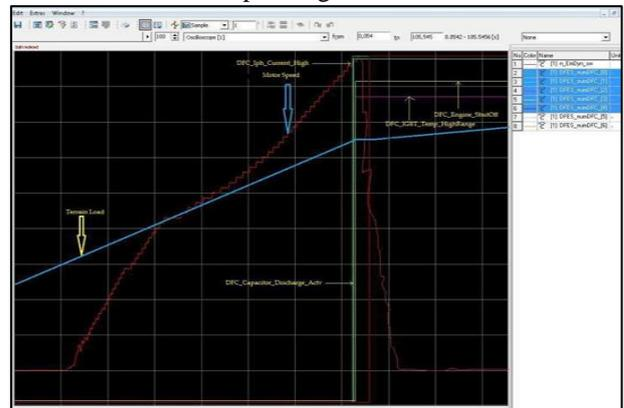
Fig. 6: Effect of Simulating Stalled motor on Inverter ECU Software
