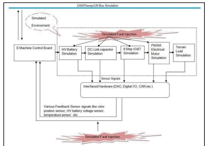
Fig. 9: Block diagram of high dynamic HIL module
