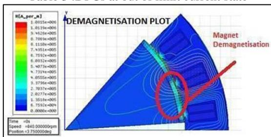
Fig. 7: Demagnetization
