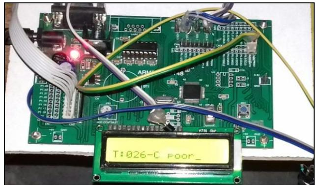
Fig. 12: LCD displaying Patient's Health Parameters
