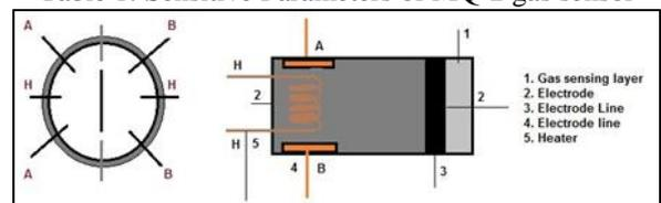
Fig. 6: Pin Configuration of MQ-2 sensor
