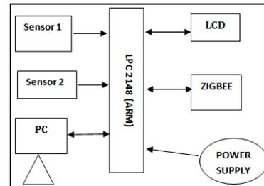
Fig. 1: Block Diagram of Home Based Station
