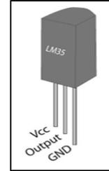
Fig. 4: LM-35 Package with Pins
