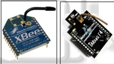
Fig. 8: Zigbee Module
