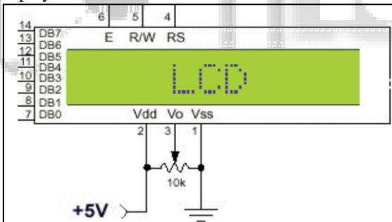
Fig. 4: Pin Diagram of LCD
