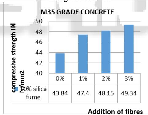
Fig. 2: Showing the variation of the compressive strength in M 35 grade concrete
