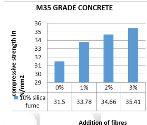
Fig. 1: Showing the variation of the compressive strength in M 35 grade concrete
