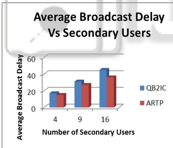
Fig. 5.2: Number of Secondary Users Vs Average Broadcast Delay
