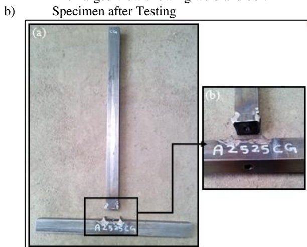
Fig. 15: (a) Photograph of Specimen A2525CG after test (b) enlarged view showing hole and bolt broken at head The breaking load is found to be 159.12 KN.
