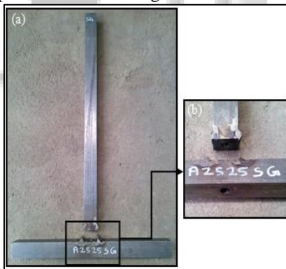
Fig. 21: (a) Photograph of Specimen A2525SG after test (b) enlarged view (c) enlarged view showing hole and bolt broken at head.
