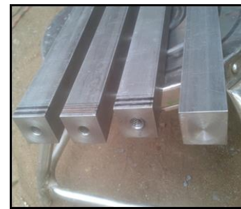
Fig. 9(a): Manufacturing of specimen (b) enlarged view of vertical bar showing tapped hole of 8mm dia.
