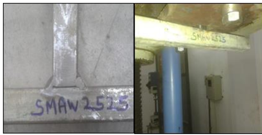
Fig. 7(a): Enlarged view of Specimen (b): Specimen SMAW2525 in the UTM before testing.
