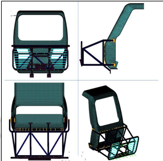
Fig. 2: describes the finite element bumper car assembly in different 2D views with different nodal structure.
