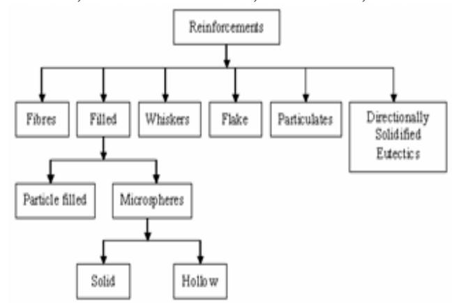
Fig. 1: Classification based on reinforcement
