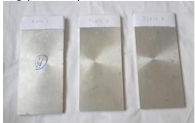
Fig. 2: Material after polishing the casted surface
